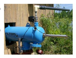
This is precisely what Marty Van Ells of Municipal Well and Pump was aiming to avoid by installing a filter in his irrigation project. Forsta self-cleaning irrigation filters provide insurance against costly landscape and turf damage, and prolong the life of sprinkler equipment. The automatic backwash cycle completely cleans the filter, eliminating the need for routine maintenance.
